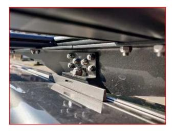
11. Insert 2 M6 bolts inside each slots of the signed crossbar and, using the M6 stop locking nuts supplied, assemble the brackets to the loading roof without completely tightening it
