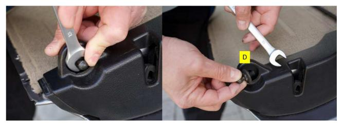
Remove the lower tailgate trim panel pulling it upwards:
