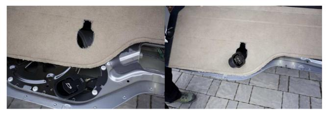
Install the handle to the bracket using the supplied M5x18 screws:
