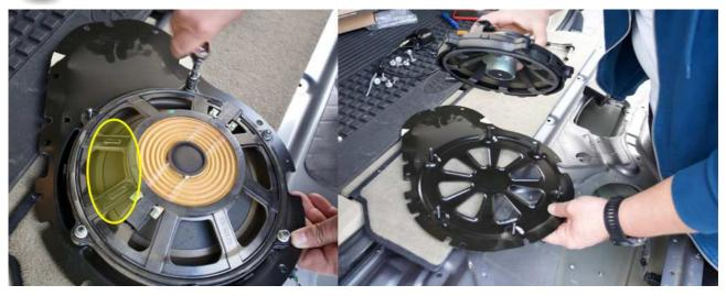
Using the angle grinder cut the subwoofer plate following the cutting line drawn earlier:
