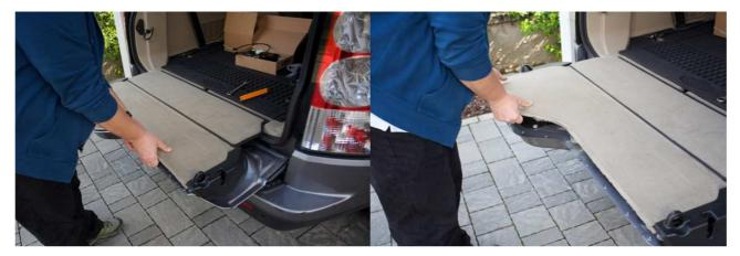
**4.2.** Subwoofer plate modifications and handle bracket installation Using T30 torx key unscrew 4 bolts (A):
