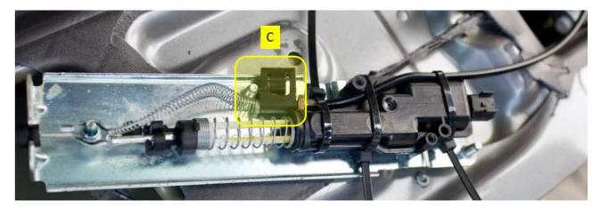
Reassemble the actuator cap then reassemble the actuator on the tailgate following the reverse procedure described in the previous paragraph 4.3:
