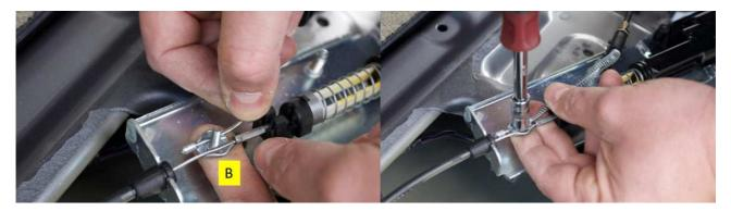
If available, put some thread locker on the joint nut. Secure the cable to the actuator as shown in the photo using the supplied cable ties:
