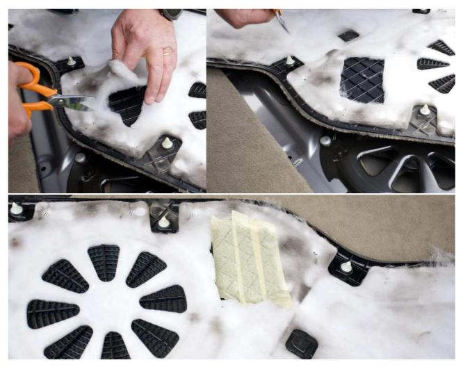
Screw the M5x50 screws (A) to the handle bracket, dirty the head of the screws with a marker, place the panel on the flap on its exact installation position and press it lightly in correspondence with the screws to mark the paper tape previously applied:
