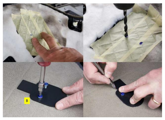
Remove the template and widen the previous 6mm holes using the 8mm bit and, using the jigsaw, cut **inside** the outline just traced:
