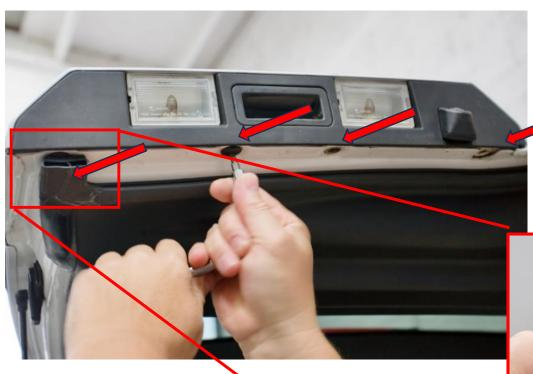
To unscrew the first bolt on the left, it is necessary to lift the rubber gasket covering it
