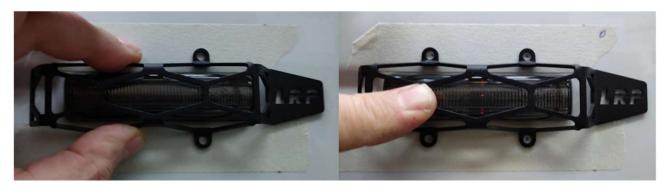
Using the drill punch, mark again the drill points. Pushing the turn light to the right and pulling it toward you, remove it from the door:
