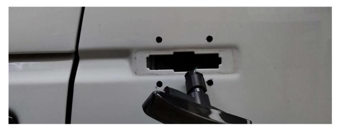
Use the rivnut tool to install provided M4 rivenuts:
