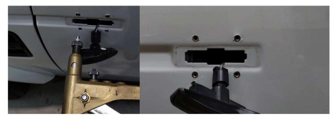
Insert in place the turn light and the 2.5 Allen key install the light guard:
