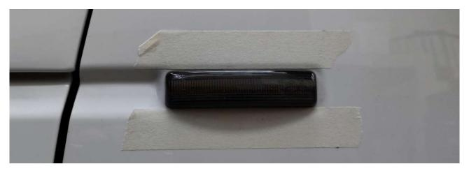
place the light guard in the center and with a pencil mark the 4 points where to make the holes:
