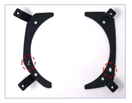
Take the bracket I and put it in place. The rounded part should be in contact with the fog lamp ring. Using 4mm bit, drill a little bit the fog light bezel to mark where to drill the holes:
