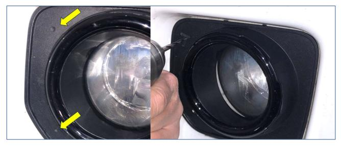
Put the bracket on place again an insert the snap rivets provided:
