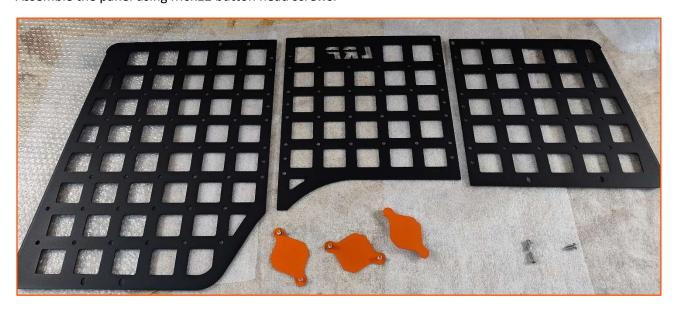
Position the magnetic device support plates "F" in according to your needs and screw them with M6 self-locking nuts:
