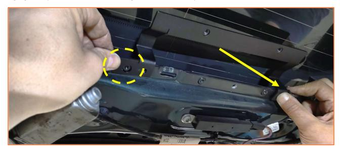
Drill holes as explained in the previous step and install the bracket using the remaining M6x14 hex head screws and self-locking nuts:
